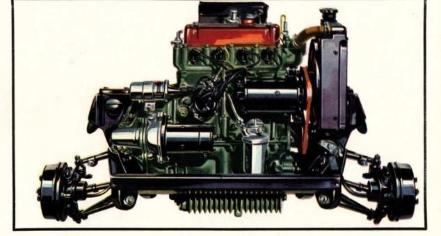
Perhaps the most revolutionary piece of automobile engineering of recent times is the amazingly compact power pack, which includes the o.h.v. 848-c.c. engine with four-speed synchromesh gearbox and final drive differential integrally built into its sump. They are assembled with front-wheel drive and independent front suspension as one extremely accessible major mechanical unit.
