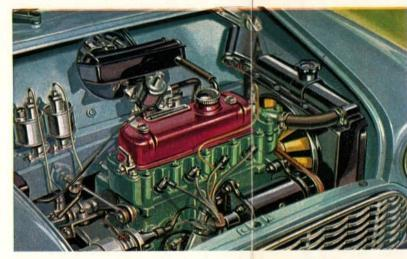
Lift the bonnet of the Austin Mini Countryman and see how the transverse installation of the power pack has helped to gain those extra-large dimensions inside the body.
