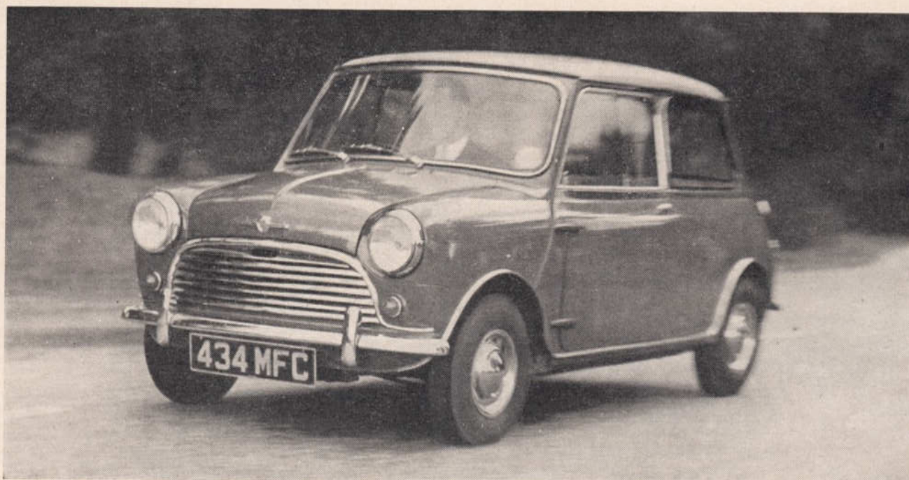
New duo-tone colour schemes, a chromium-plated grille and the Morris Cooper motif are the only exterior features which distinguish this from standard Mini-Minors.
