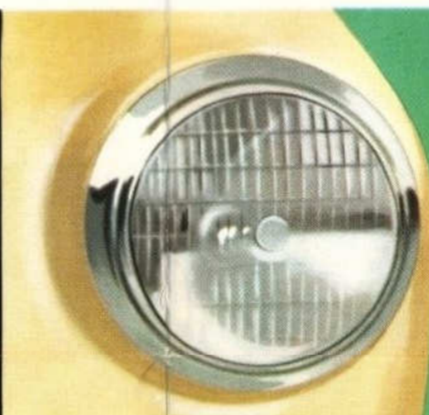
12-volt headlamps are fitted with dippers. Separate flashing direction indicators are standard equipment.
