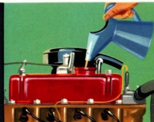
Servicing is three times as easy—the same oil and filler are used for engine, gears, and axle.
