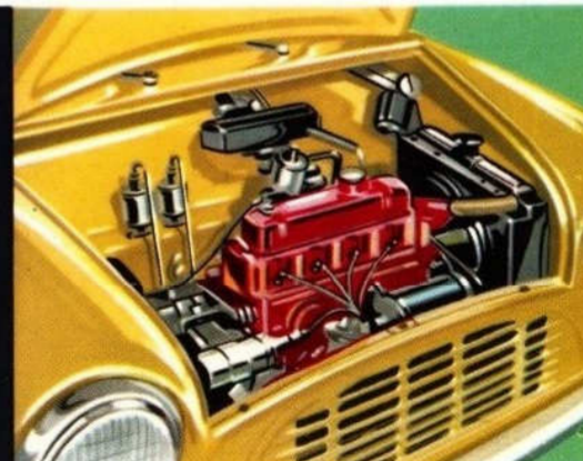
'East-West' engine combined with clutch, gears, and drive axle in one unit.
