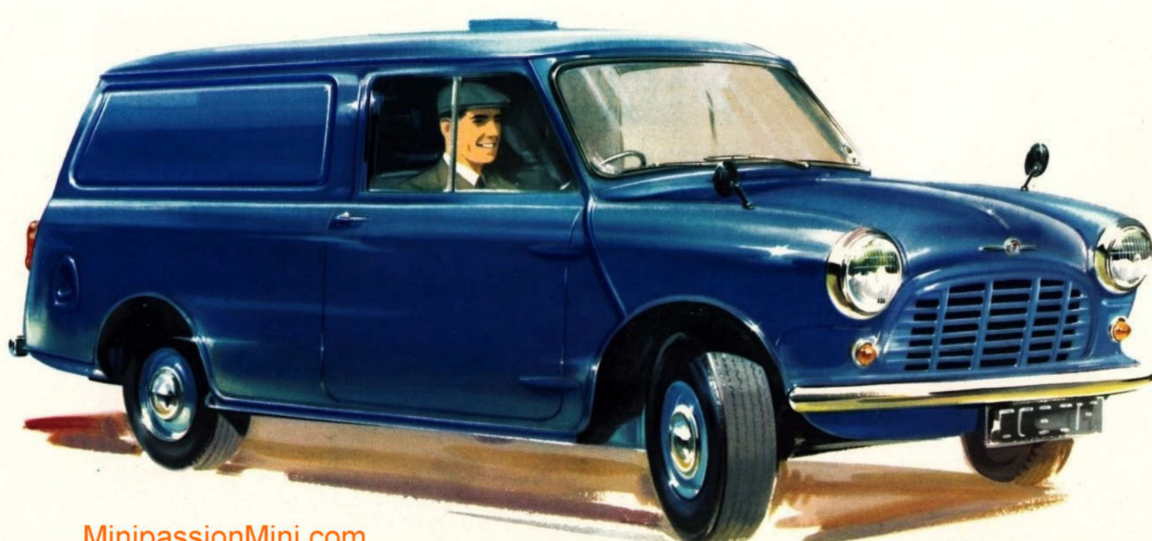
Draught-free door windows slide open and shut—extraction ventilator provided in roof.
